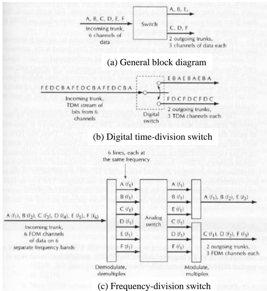
Example of digital versus analog switching
